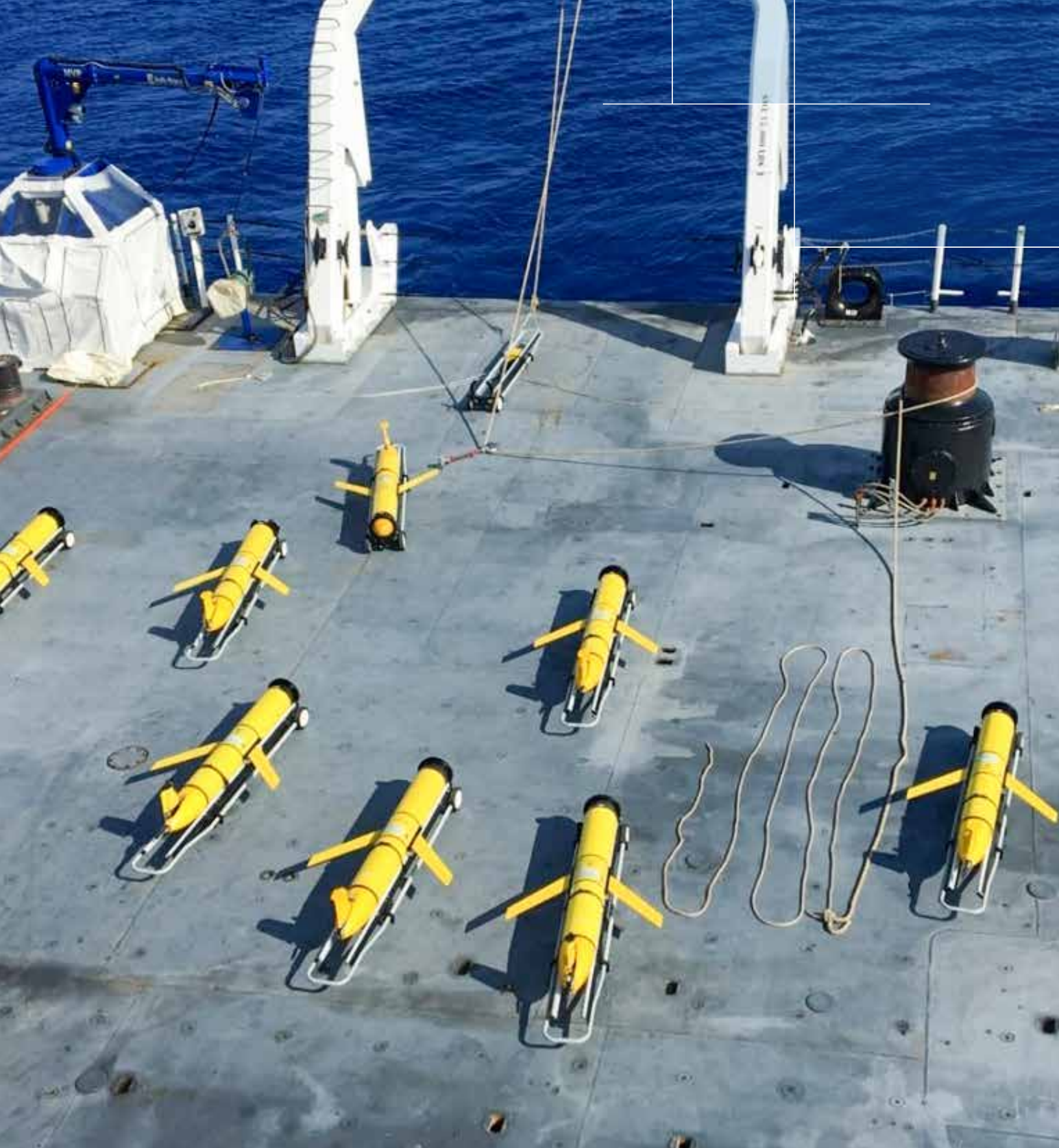
A full complement of unmanned LBS Gliders are readied for deployment from a T-AGS Oceanographic Survey Ship. Once launched they will support the collection of oceanographic environmental data for up to 90 days.
