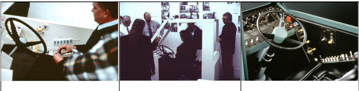
Figure 2. On the left, Sergeant Coker considers changing the location of several user interface controls within the context of a full-size cab mockup covered in Velcro. The photo in the middle shows that the meeting with Sergeant Coker took place with all the project stakeholders standing around the Velcro-model. On the right is the final appearance model of the redesigned cab.
