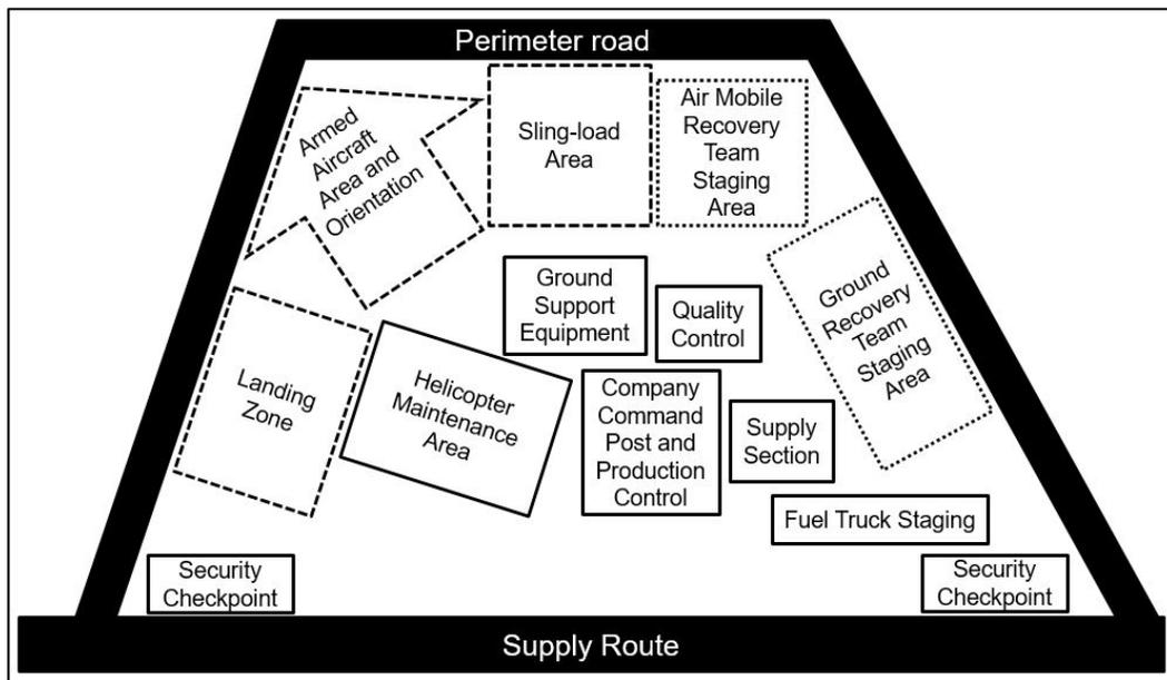
**Figure 2-4. Helicopter maintenance collection point**
