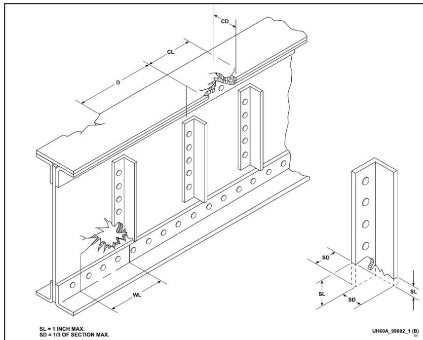
**Figure 2-2. Inspecting damage to aircraft airframe**
