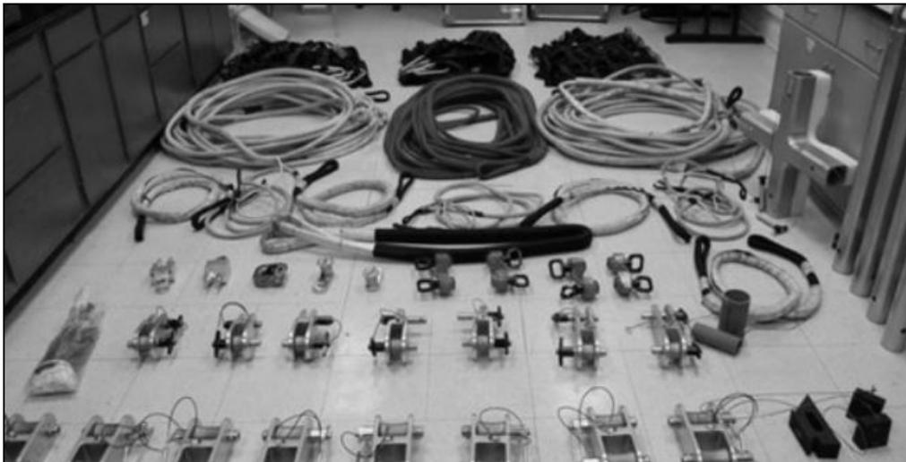
**Figure C-5. Unit maintenance aerial recovery kit**
