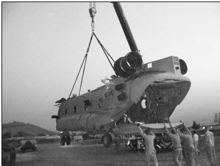
**Figure 3-3. Recovery by crane**
