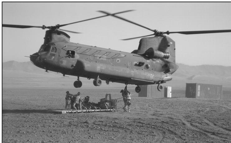
**Figure 3-4. Recovering aircraft components**
