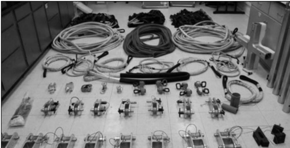
**Figure C-5. Unit maintenance aerial recovery kit**
