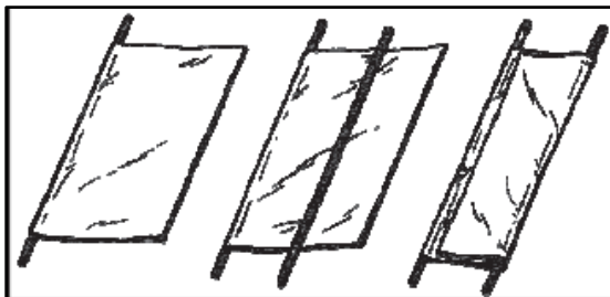
Figure 3-14. Litter made with blankets and poles
