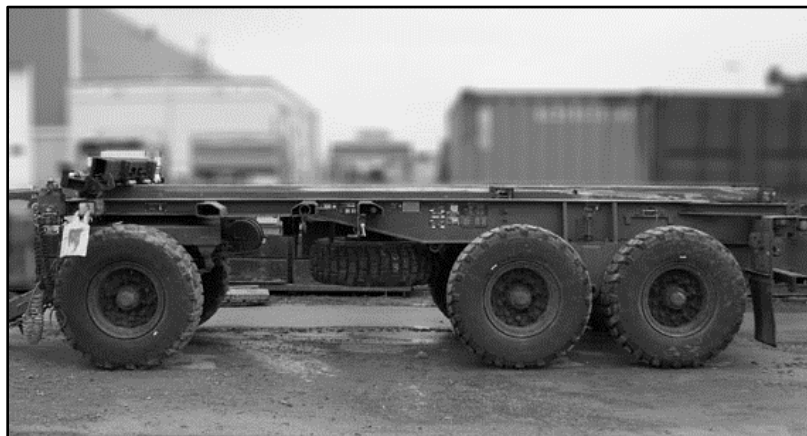
Figure 4-6. M1075A1, Palletized Load System
