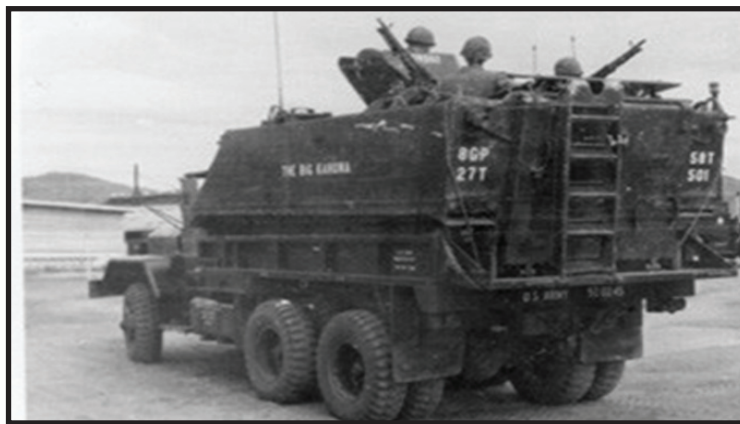
Figure 14. The Big Kahuna . APC hull mounted in a 5-ton truck.
